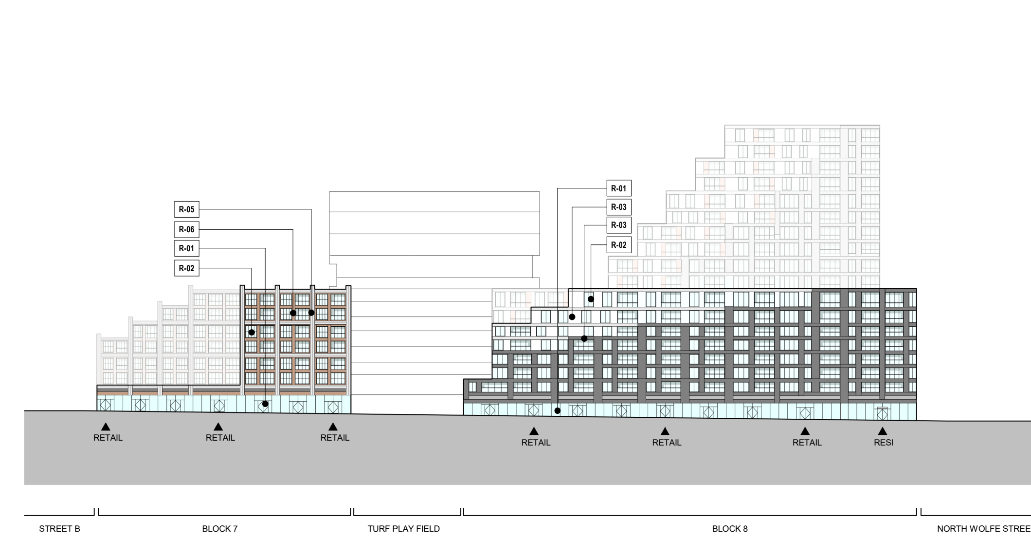
3 NORTH ELEVATION - STREET 3 SCALE: 1/8" = 1'-0"
